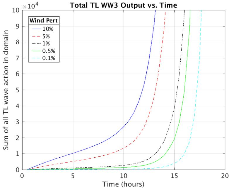
Figure 9. Sum of all TL wave action in model domain plotted versus time for five separate simulations, each of which used a different wind perturbation.
