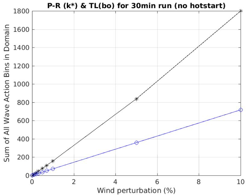
Figure 11. Comparison of total energy density output (TL WW3 and perturbed-minus-unperturbed WW3) plotted versus wind forcing perturbation size. Unlike Figure 2, *these simulations did NOT use a restart (hotstart) file to begin from an authentic ocean state.*, which led to a nearly uniform P-U trend for all perturbation sizes (compare to Figure 3). Model run time was 30 minutes.
