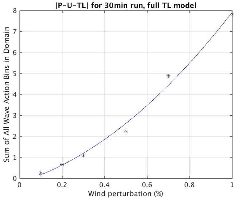
Figure 6. Absolute difference of total wave action (perturbed-minus-unperturbed minus TL), plotted versus wind forcing perturbation size after **30-min** simulation, smaller perturbations only. Best-fit curve (blue line) follows polynomial  $y = 4.98x^2 + 3.14x - 0.2$ . RMS error of data points is 0.25. Normalized by the curve value at 1% wind perturbation, this is 0.032.
