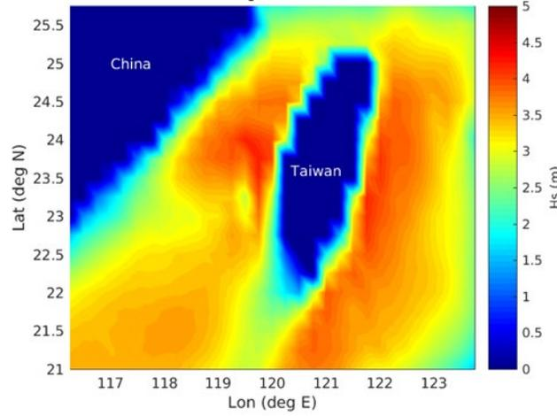
Figure 2. Model test domain (South China Sea region), including model-estimated significant wave height values for a single timestep in January 2021. To facilitate testing of model’s wave-ice interaction component, an idealized “iceberg” was inserted into the domain at approximately 118°E, 23°N.
