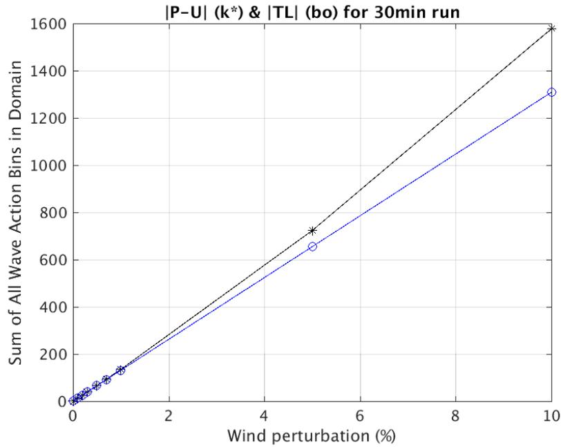
Figure 3. Comparison of total energy density output (TL WW3 and perturbed-minus-unperturbed WW3) plotted versus wind forcing perturbation size. Model run time was **30 minutes**.
