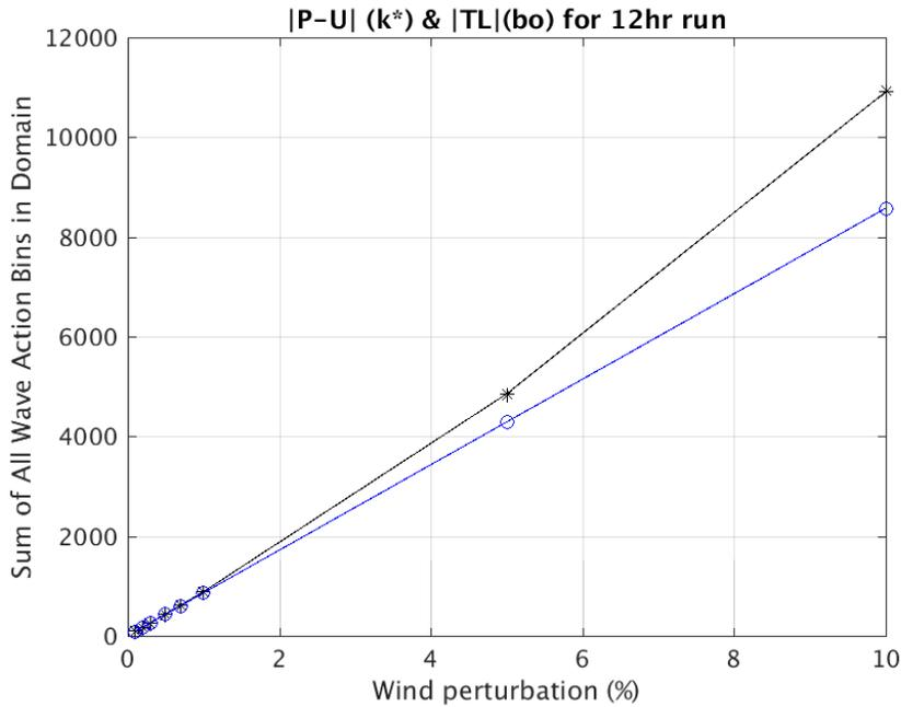
Figure 5. Comparison of total energy density output (TL WW3 and perturbed-minus-unperturbed WW3) plotted versus wind forcing perturbation size. Model run time was **12 hours**.
