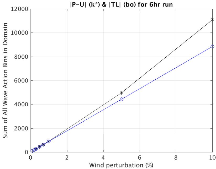
Figure 4. Comparison of total energy density output (TL WW3 and perturbed-minus-unperturbed WW3) plotted versus wind forcing perturbation size. Model run time was **6 hours**.
