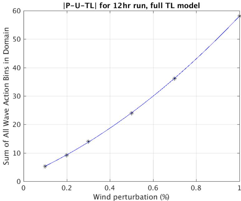
Figure 8. Absolute difference of total wave action (perturbed-minus-unperturbed minus TL), plotted versus wind forcing perturbation size after **12-hr** simulation, smaller perturbations only. Best-fit curve (blue line) follows polynomial  $y = 23.46x^2 + 32.8x + 1.81$ . RMS error of data points is 0.11. Normalized by the curve value at 1% wind perturbation, this is 0.002.
