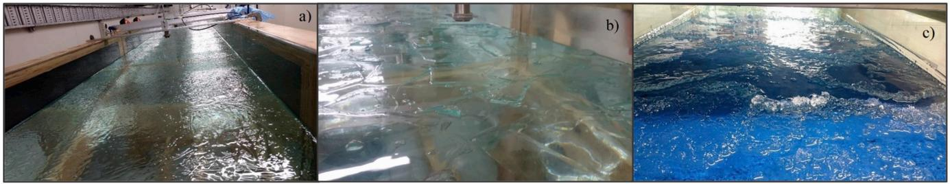
Fig. 1. Types of manufactured ice for the experiments: a) sheet ice, b) ice floes, and c) grease ice.
