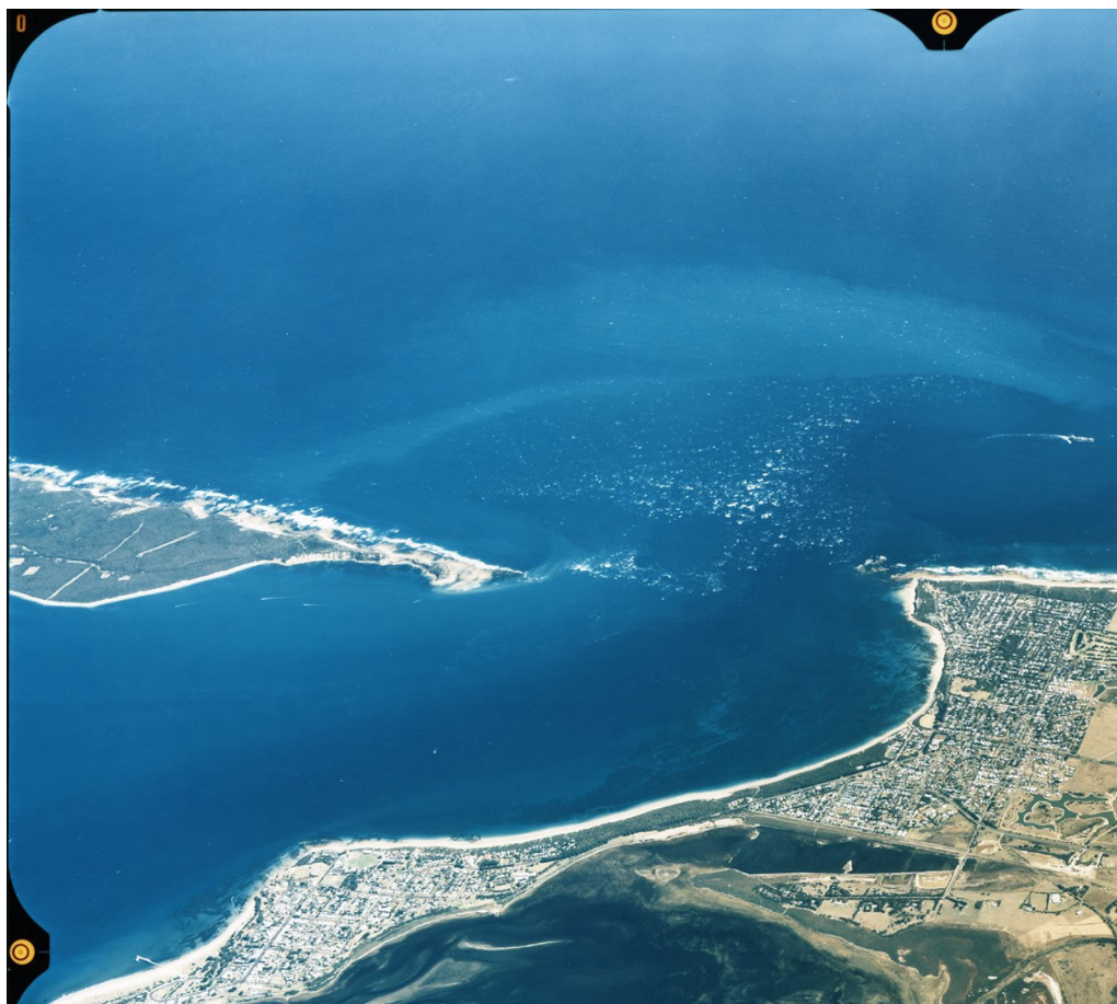
Figure 3. Aerial photograph of Port Phillip Heads showing wave breaking induced by ebb currents. The image was kindly provided by the Port of Melbourne Corporation.
