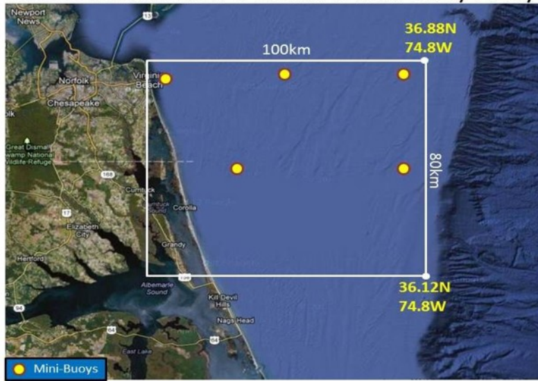
Figure 4: Domain boundaries for SWANFAR ® stationary assimilation. Approximate locations of Scripps mini-buoys are marked as yellow circles.
