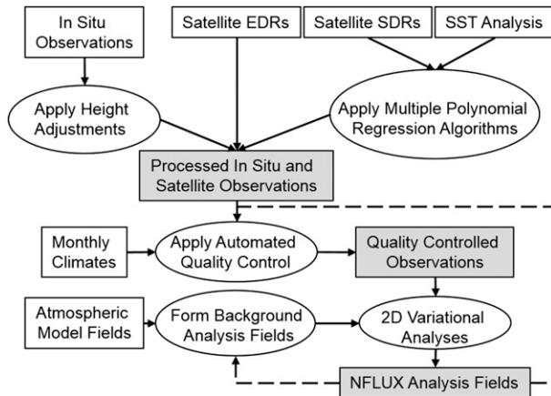
FIG. 1. The NFLUX system data-flow schematic. Unshaded rectangles signify the input datasets, ovals signify major internal processes, and shaded rectangles signify the end product from each primary component of the NFLUX system. The dashed arrow lines indicate that the end product from one cycle is used in the following cycle.
