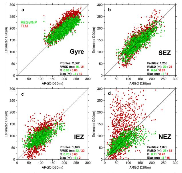
**Fig. 10.** Regional D20 scatter plots of the REGWNP (green) and TLM (red) against Argo observations for the (a) Gyre, (b) SEZ, (c) IEZ, and (d) NEZ. The Argo profiles compared are from May–October of 2009–2010 (blue dots in Fig. 1a). Sample number, RMSD, correlation and bias with respect to Argo are shown. (For interpretation of the references to color in this figure legend, the reader is referred to the web version of this article.)
