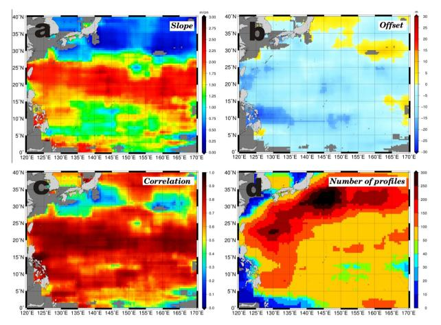
**Fig. 4.** The spatial distribution of (a) the slope and (b) the offset of the Eq. (2) for D20 in September. (c) The spatial distribution of the correlation between D20 and SSHA. (d) The number of profiles used for developing the regression at each 0.25° × 0.25° grid point. Grey areas represent the significance level <99%.
