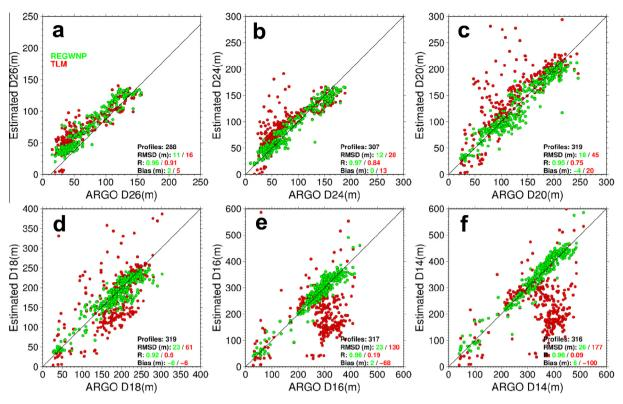
**Fig. 15.** Comparisons of (a) D26, (b) D24, (c) D20, (d) D18, (e) D16 and (f) D14 between the REGWNP (green dots) and TLM (red dots) and Argo observations in September of 2010. D24, D18, D16 and D14 are obtained by interpolation or extrapolation for the TLM. Sample number, RMSD, correlation and bias with respect to Argo are shown. (For interpretation of the references to color in this figure legend, the reader is referred to the web version of this article.)
