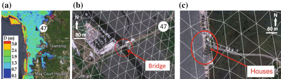
Fig. 9 A zoom view of the hydrodynamic prediction of flooding in Scenario 4 at residence zones and transportation systems within the region marked by the red rectangle in Fig. 6a. Houses are marked as red arrows, bridges are marked as red circles, and these in b and c are located near Middle Township in a . a Local flooded region, b mesh at a bridge, c mesh at houses
