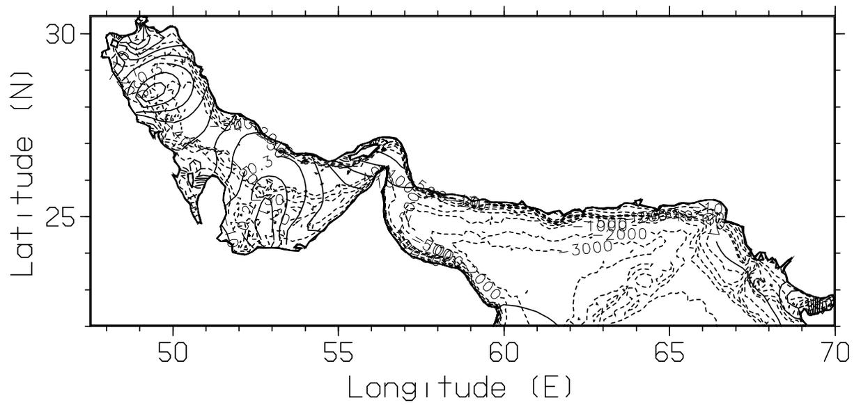
Fig. 5 — NAVO Persian Gulf domain, bathymetry in m (dashed line), M<sub>2</sub> tidal amplitude from OTIS in m (solid line).
