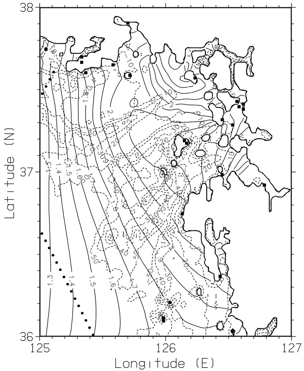
Fig. 9 — Incheon, Korea domain, bathymetry in m (dashed line), M<sub>2</sub> tidal amplitude from OTIS in m (solid line), and locations of IHO stations (squares), and TIL data (dots) used for computing errors.
