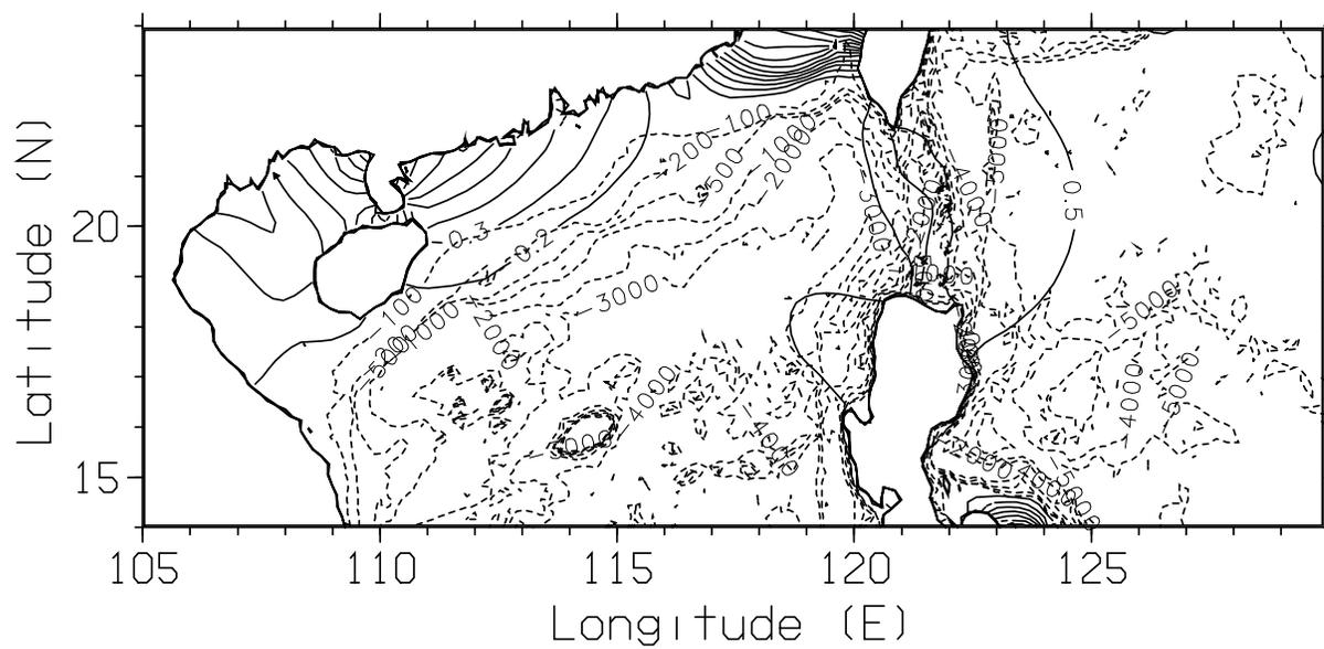
Fig. 4 — NAVO South China Sea domain, bathymetry in m (dashed line), M<sub>2</sub> tidal amplitude from OTIS in m (solid line).
