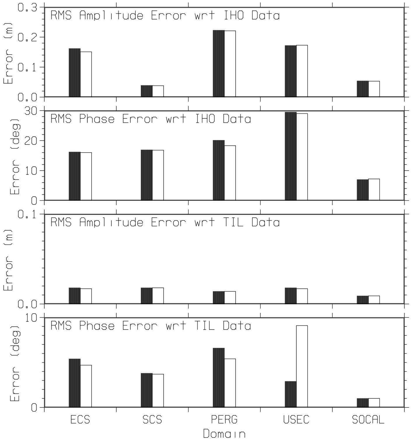
Fig. 17 — Comparison of RMS errors for OTIS with assimilation of the PF altimeter data (black bars) and the NRL altimeter data (white bars) for the five NAVO domains.
