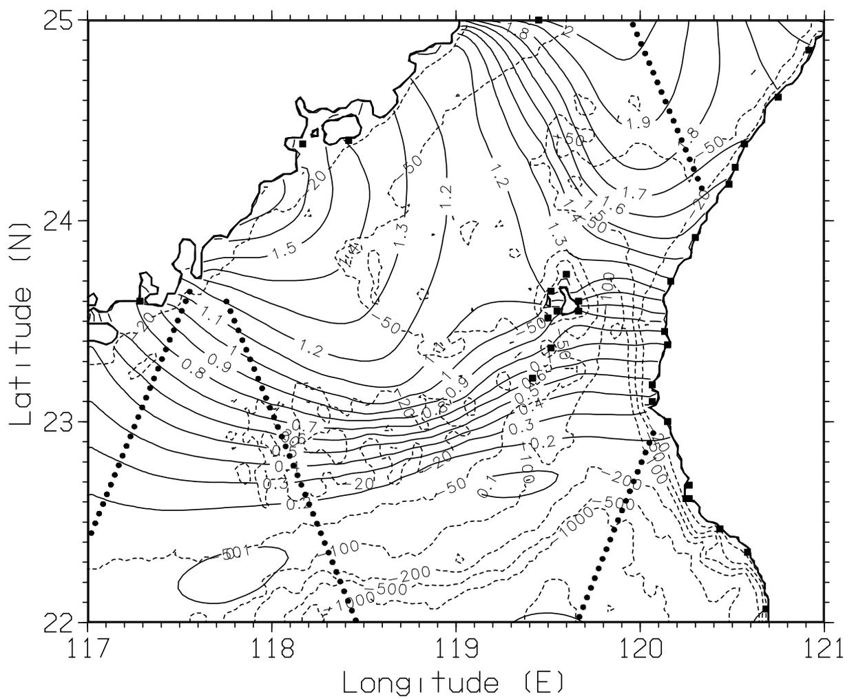
Fig. 11 — Taiwan Strait domain, bathymetry in m (dashed line),  $M_2$  tidal amplitude from OTIS in m (solid line), and locations of IHO stations (squares), and TIL data (dots) used for computing errors.
