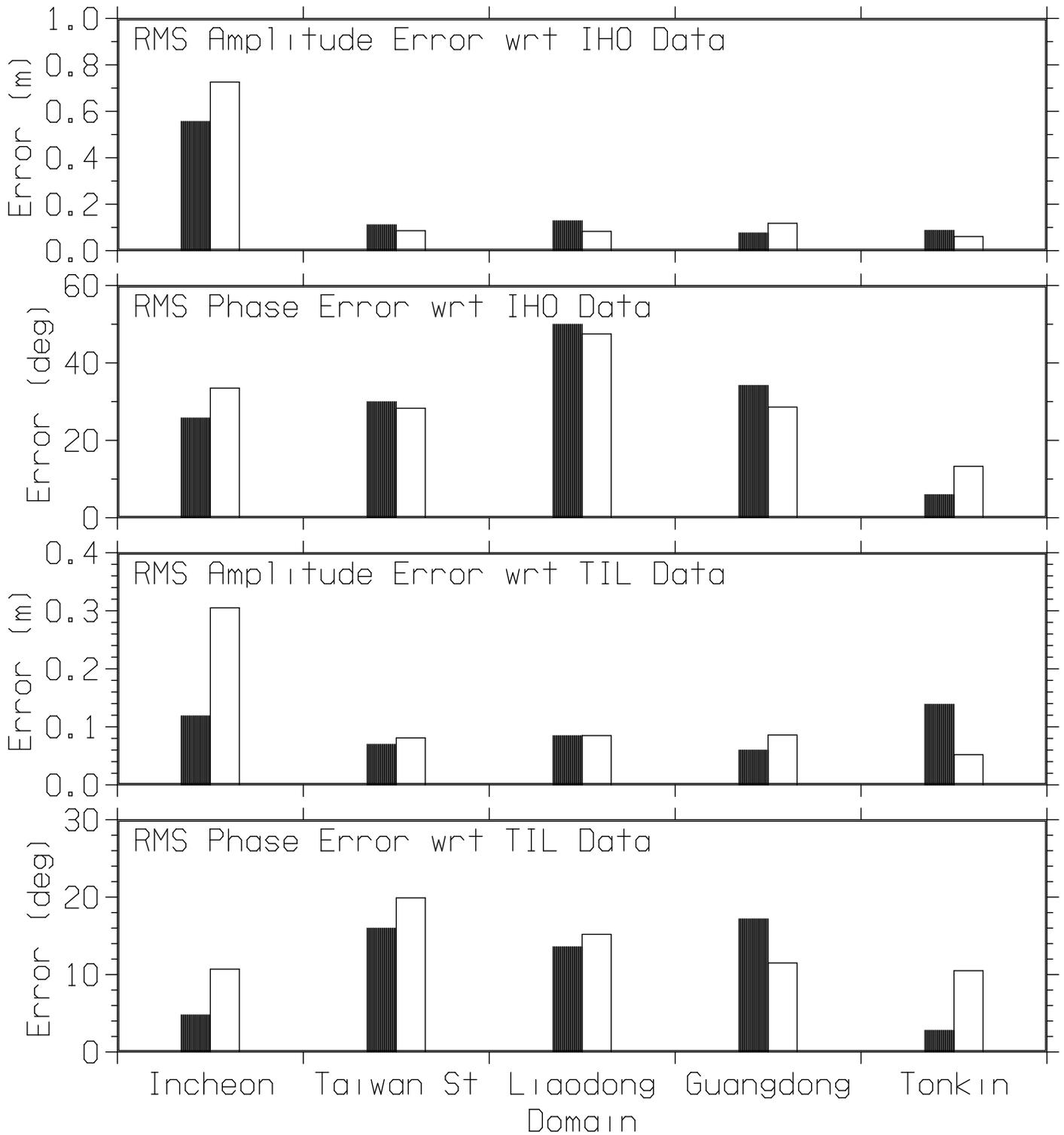
Fig. 21 — Comparison of RMS errors for NCOM with BCs from a local OTIS analysis (black bars) and from a tidal simulations with PCTides (white bars).
