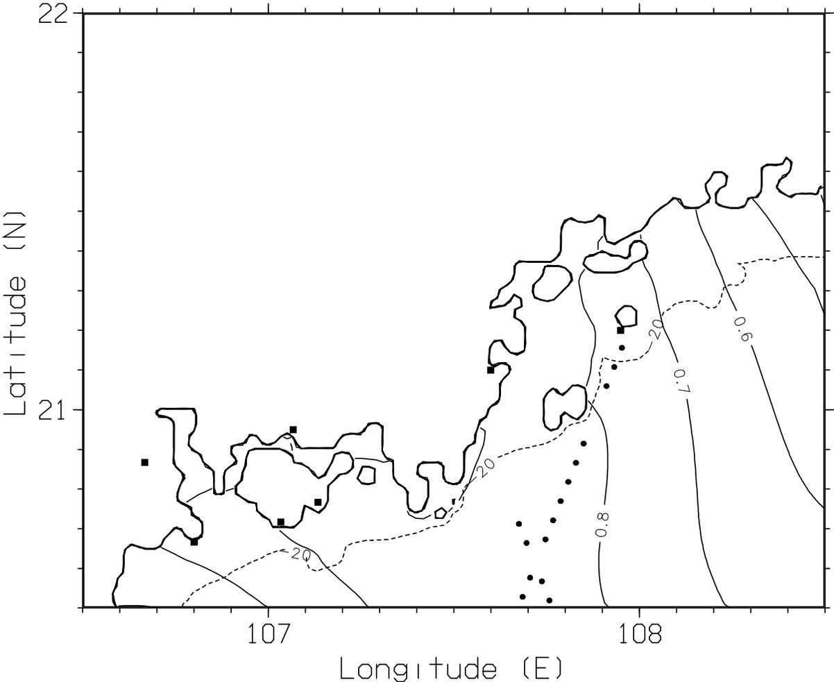
Fig. 14 — Gulf of Tonkin domain, bathymetry in m (dashed line),  $O_1$  tidal amplitude from OTIS in m (solid line), and locations of IHO stations (squares), and TIL data (dots) used for computing errors.
