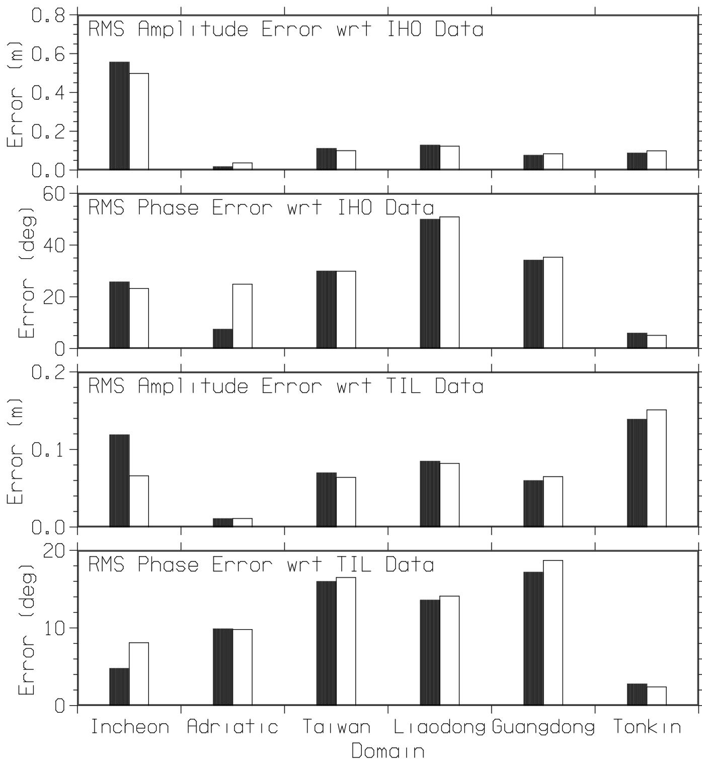
Fig. 20 — Comparison of RMS errors for NCOM with BC from OTIS with assimilation of the PF altimeter data (black bars) and the NRL altimeter data (white bars) for the Incheon, Adriatic, Taiwan St., Liaodong Bay, Guangdong, and Tonkin Gulf domains.
