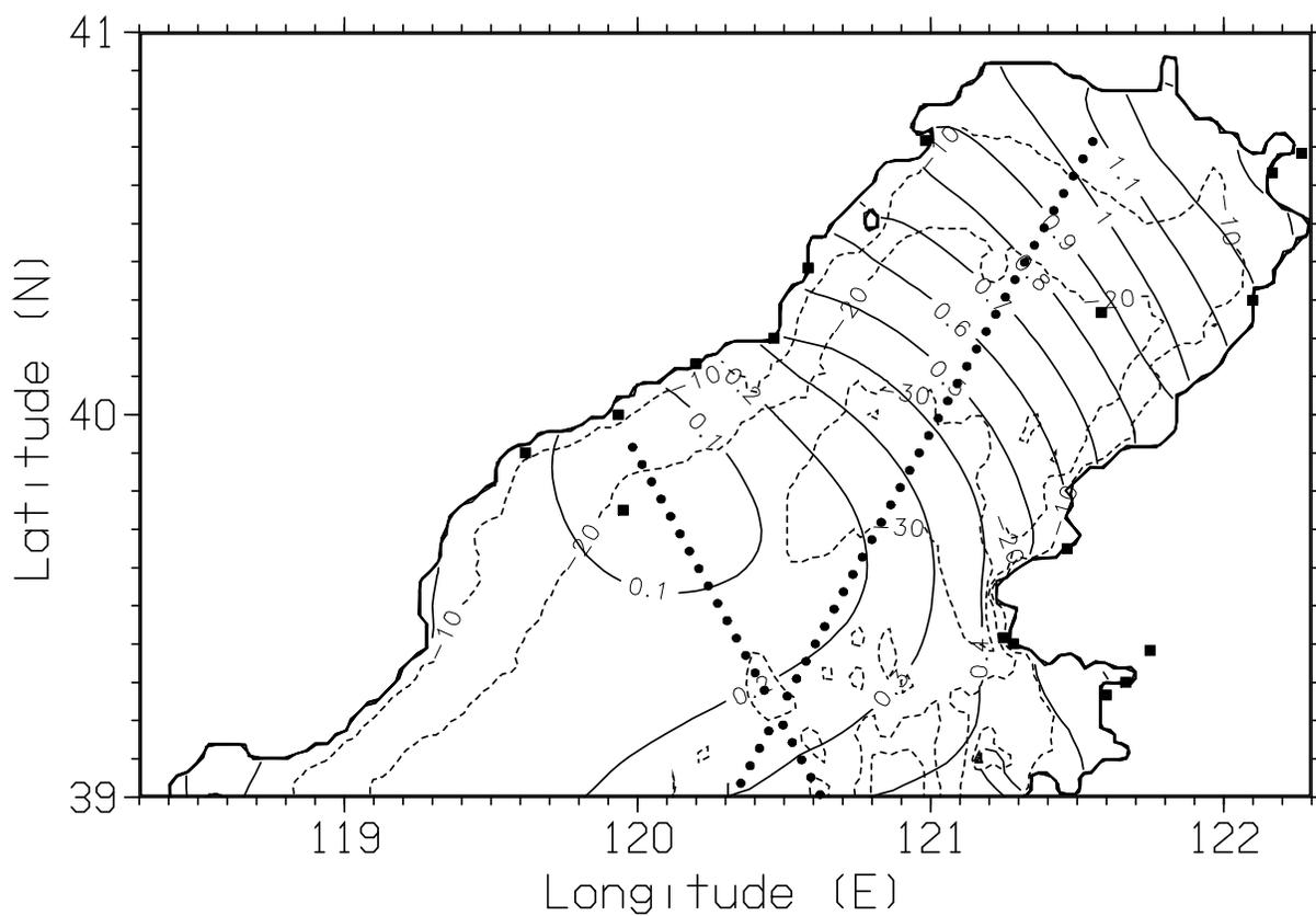
Fig. 12 — Liaodong Bay domain, bathymetry in m (dashed line),  $M_2$  tidal amplitude from OTIS in m (solid line), and locations of IHO stations (squares), and TIL data (dots) used for computing errors.
