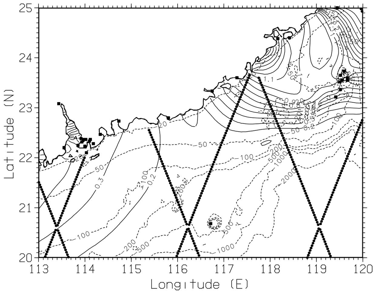
Fig. 13 — Guangdong, China domain, bathymetry in m (dashed line),  $M_2$  tidal amplitude from OTIS in m (solid line), and locations of IHO stations (squares), and TIL data (dots) used for computing errors.
