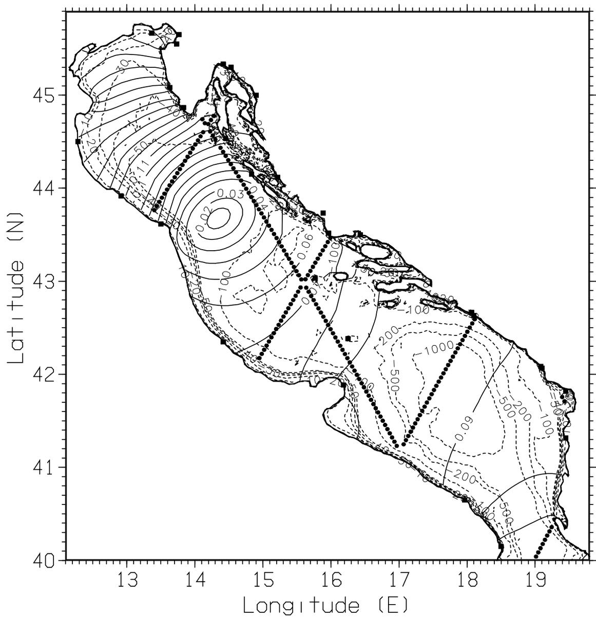
Fig. 10 — Adriatic Sea domain, bathymetry in m (dashed line),  $M_2$  tidal amplitude from OTIS in m (solid line), and locations of IHO stations (squares), and TIL data (dots) used for computing errors.
