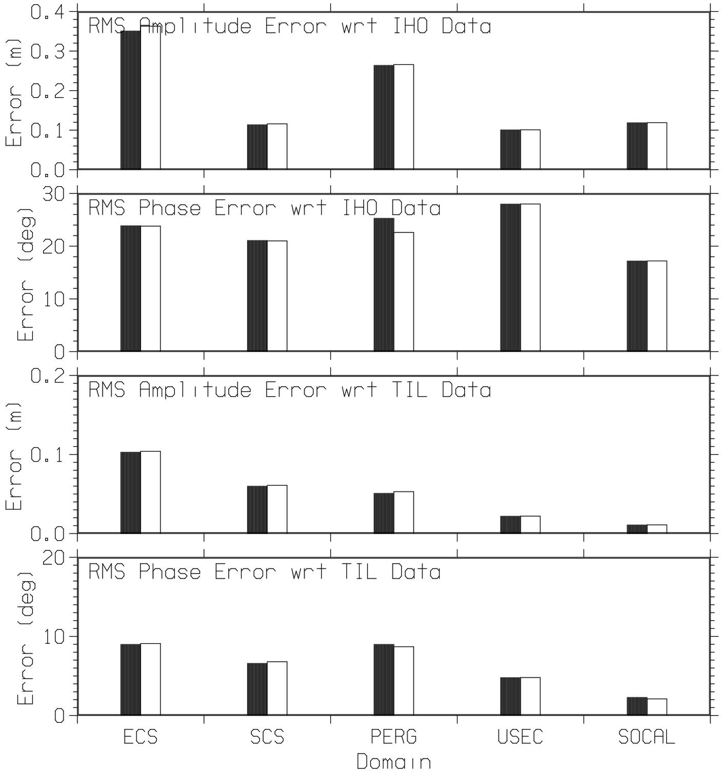
Fig. 18 — Comparison of RMS errors for NCOM with BC from OTIS with assimilation of the PF altimeter data (black bars) and the NRL altimeter data (white bars) for the five NAVO domains.
