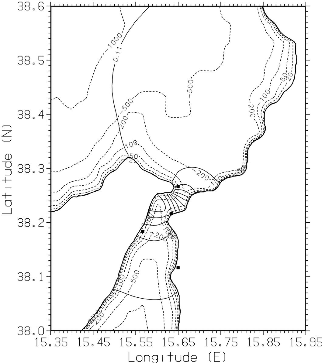
Fig. 15 — Messina Strait domain, bathymetry in m (dashed line),  $M_2$  tidal amplitude from OTIS in m (solid line), and locations of IHO stations (squares), and TIL data (dots) used for computing errors.
