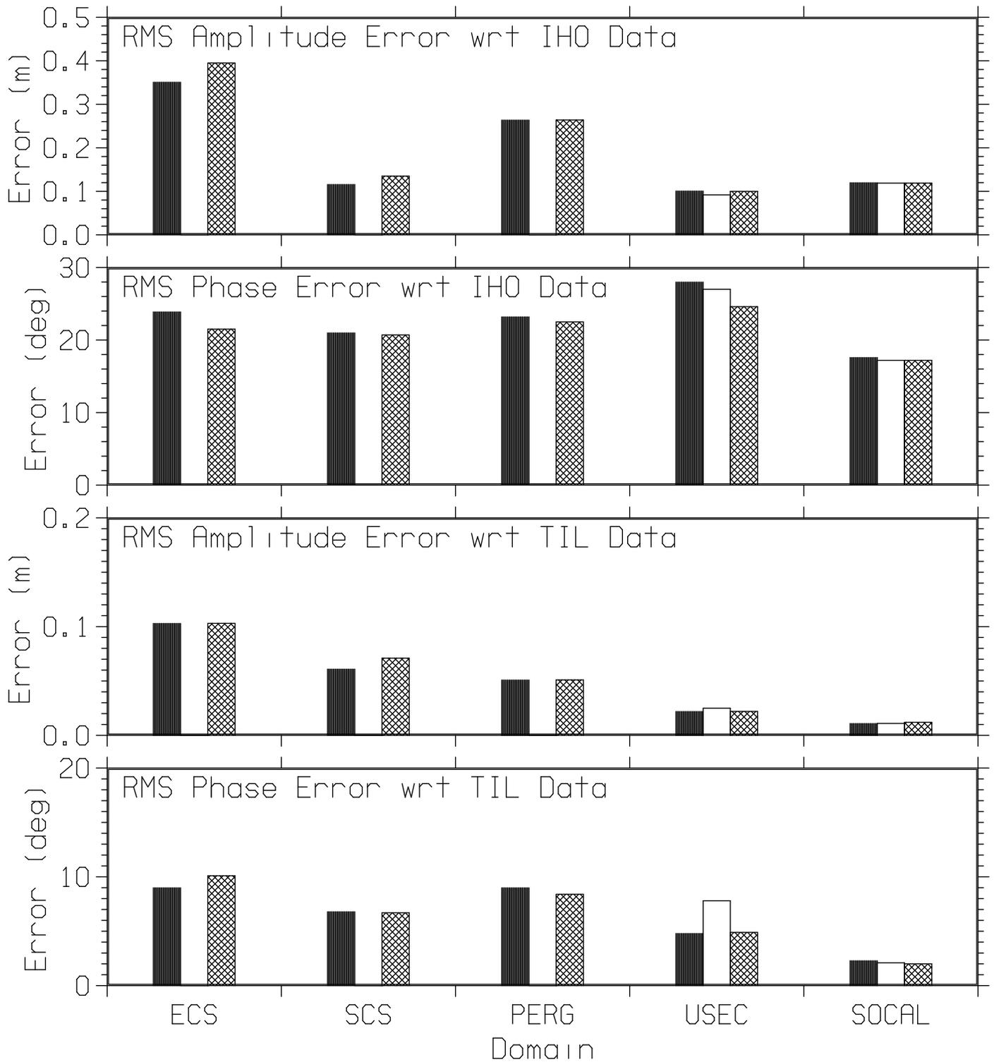
Fig. 8 — Comparison of  $M_2$  RMS tidal errors for NCOM with BCs from a local OTIS analysis (black bars), an OSU regional tidal DB (white bars), and the OSU Global tidal DB (cross-hatched bars) for the five NAVO regional domains.
