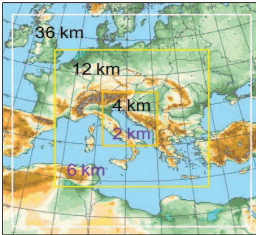
Fig. 1: Atmospheric and ocean grid setup for the Adriatic Sea. The resolution for the atmospheric nests (black) and the ocean nests (purple) are indicated.
