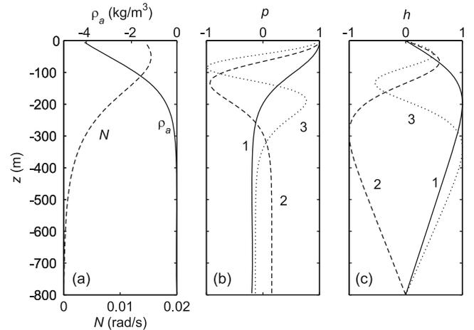
**Figure 1.** (a) Density  $\rho_a$  in  $\text{kg m}^{-3}$  and buoyancy frequency  $N$  in  $\text{rad s}^{-1}$  in Experiments 1 and 2. The corresponding normal modes are shown (b) for horizontal velocity and (c) for density perturbation. The phase speeds are  $1.52$ ,  $0.64$ , and  $0.41 \text{ m s}^{-1}$  for the first three modes.
