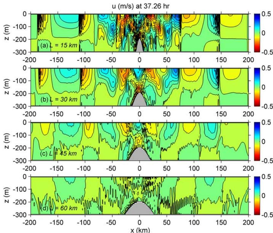
**Figure 6.** Contour plots of  $u$  velocity at slack water before flood tide at  $t = 37.26$  hours for four scale widths of the ridge ( $L$ ): (a) 15 km, (b) 30 km, (c) 45 km, and (d) 60 km. The contour interval is  $0.05 \text{ m s}^{-1}$ .
