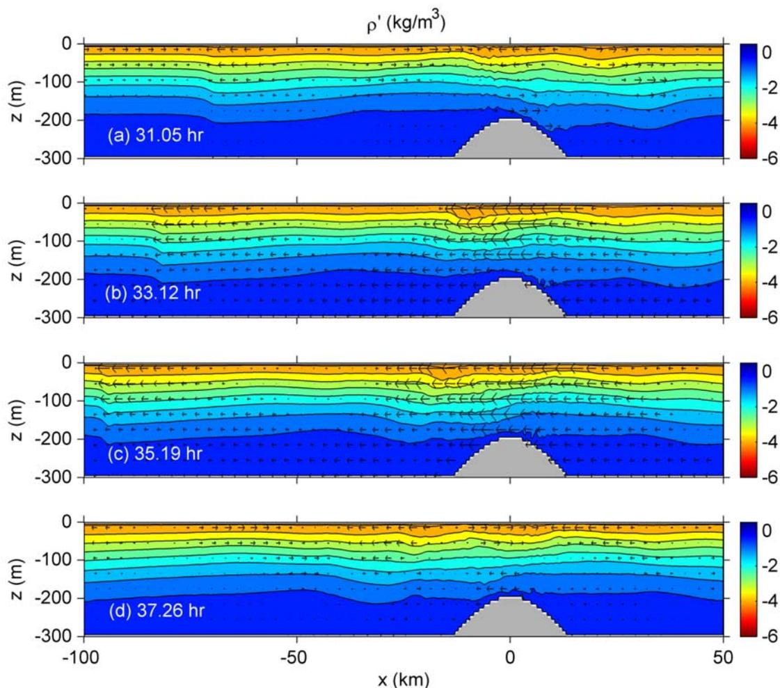
**Figure 3.** Contour plot of perturbation density ( $\rho'$ ) in  $\text{kg m}^{-3}$  for Experiment 1b at (a) 31.05, (b) 33.12, (c) 35.19, and (d) 37.26 hours during the flood tide. The contour interval is  $0.5 \text{ kg m}^{-3}$ . The maximum velocity is  $0.5 \text{ m s}^{-1}$  for  $u$  and  $0.01 \text{ m s}^{-1}$  for  $w$ .
