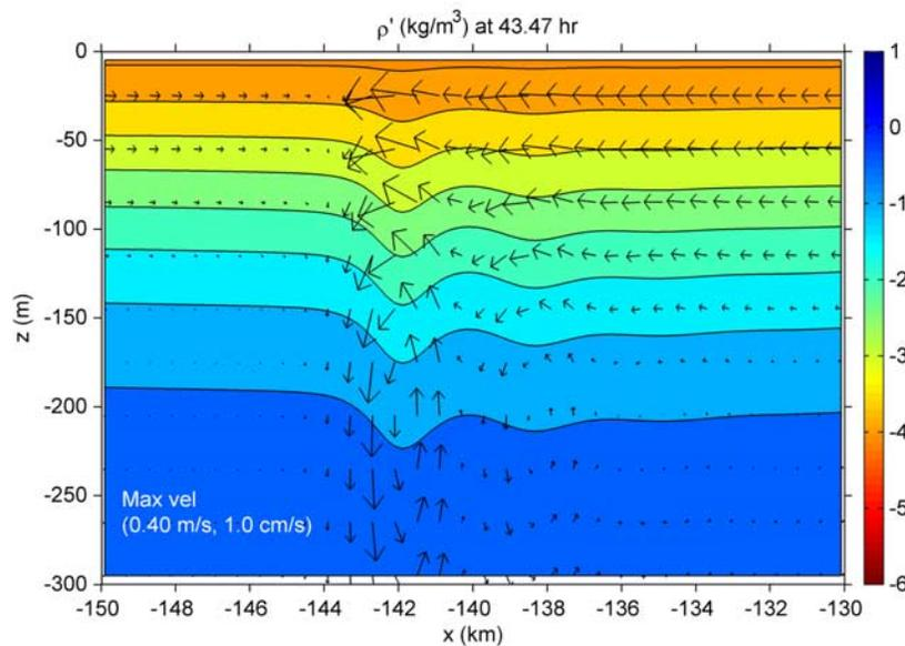
**Figure 4.** Perturbation density contours and the velocity vector in the  $x$ - $z$  plane, showing a well-developed solitary wave train at 43.47 hours in Experiment 1b. Contour values are from  $-4$  to  $-0.5 \text{ kg m}^{-3}$  at a contour interval of  $0.5 \text{ kg m}^{-3}$ . The maximum velocity is  $0.4 \text{ m s}^{-1}$  for  $u$  and  $0.01 \text{ m s}^{-1}$  for  $w$ .
