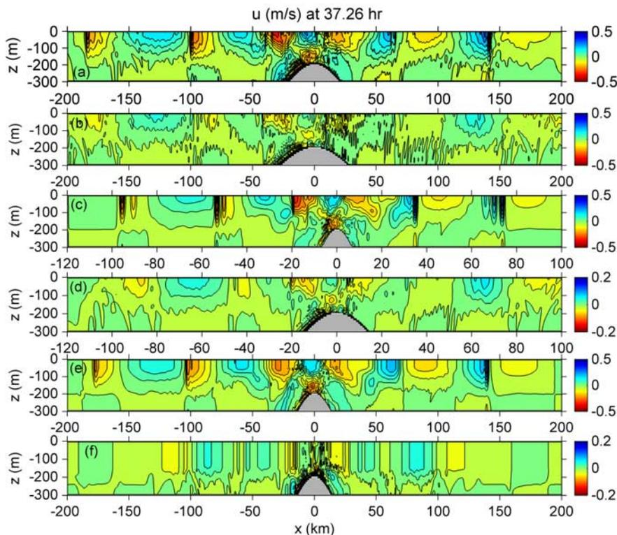
**Figure 7.** Contour plots of  $u$  velocity at slack water before flood tide at  $t = 37.26$  hours for (a) Experiment 2a, (b) Experiment 2b, (c) Experiment 3a, (d) Experiment 3b, (e) Experiment 4a, and (f) Experiment 4b. The contour interval is  $0.05 \text{ m s}^{-1}$  in all cases except  $0.02 \text{ m s}^{-1}$  in Figures 7d and 7f.
