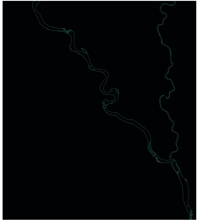
Fig. 5. Water edges as determined by a Laplace edge finding filter.
