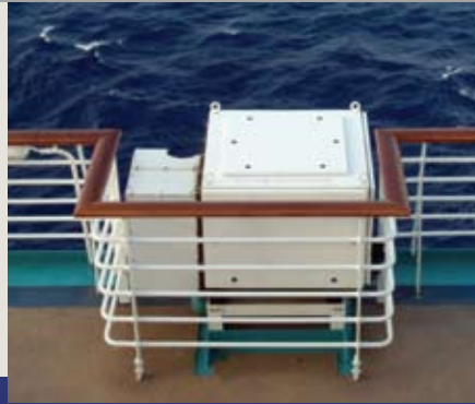
The Marine-Atmospheric Emitted Radiance Interferometer (M-AERI), which accurately measures the ocean's skin temperature. Credit: Hunter Augustus, University of Miami, Rosenstiel School of Marine and Atmospheric Science
