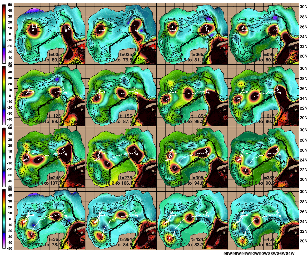
Figure 14. Temporal variation in SSH (cm) from the GOM model using HYCOM (see text for model details). SSH is depicted every 30 days starting 5 January 2000 for 450 model days. Trajectory of the center of eddies L1 and L2 are marked with white dots and lines every 10 days.
