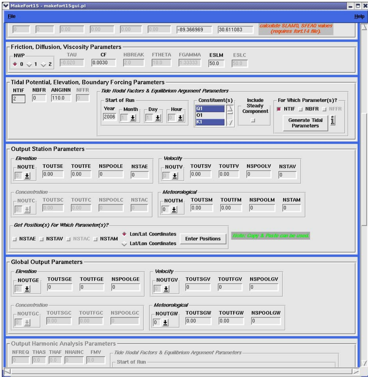
Figure 11. GUI features include a) the selection of non-adjacent list items shown by the highlighted “Constituents” “Q1” and “K1”, b) radio buttons for selecting parameter values as evidenced by the selection of NWP = 0 under the Friction, Diffusion, Viscosity Parameters panel and, c) the enabling and disabling of checkboxes evident for NTIF and NBFR, respectively.
