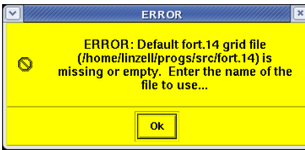
Figure 7. The ERROR popup issued if a fort.14 grid file needed but not found.
