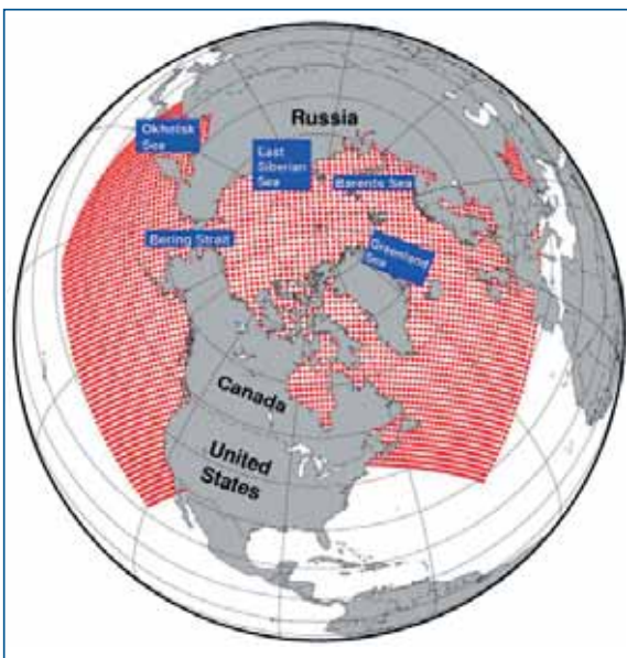
Figure 3 — Polar Ice Prediction System (PIPS 2.0) model domain and grid: every fourth point is plotted.
