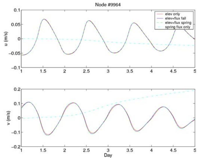
Fig. 15. Pearl River E-W and N-S velocity components at station #9964 for three forcing conditions in spring and one in fall.
