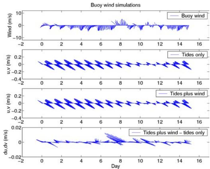
Fig. 6. Sensitivity to wind forcing. 1) NDBC Buoy 42007 winds May 15-29, 2001; 2) computed currents forced by tides only; 3) computed currents forced by tide and wind stress; 4) currents from 3) minus the currents from 2).
