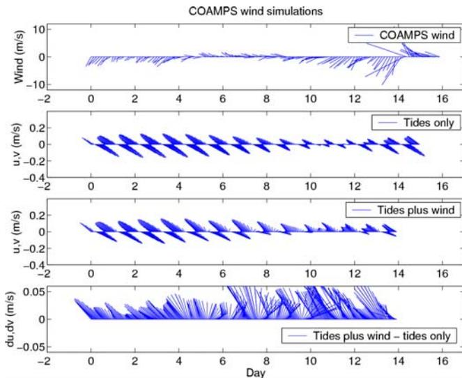
Fig. 5. Sensitivity to wind forcing. 1) COAMPS winds May 15-29, 2001; 2) computed currents forced by tides only; 3) computed currents forced by tide and wind stress; 4) currents from 3) minus the currents from 2).
