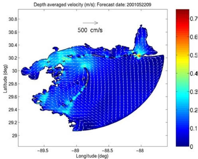
Fig. 7. ADCIRC computed currents on May 22, 2001 09Z forced by NDBC buoy winds and tides. Current magnitudes are contoured; directions are indicated by the arrows.
