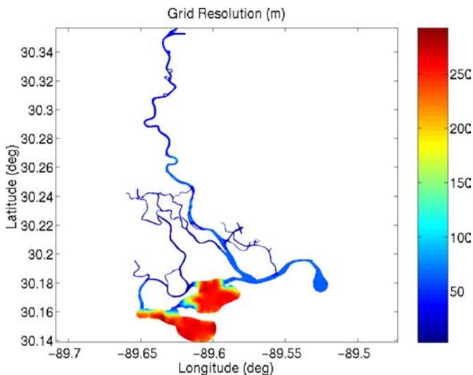
Fig. 4. Resolution of the Pearl River model grid. The range is 3 to 275 m.
