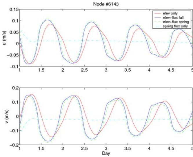
Fig. 12. Pearl River E-W and N-S velocity components at station #6143 for three forcing conditions in spring and one in fall.
