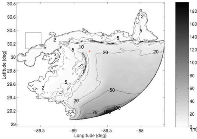
Fig. 1. Bathymetry of the Mississippi Bight domain. Contours are shown at 2, 5, 10, 20, 50, 100, and 150 m. The location of NDBC buoy 42007 is depicted by an asterisk (\*). The location of the Pearl River model is identified by the bounding box in the NW corner of the domain.
