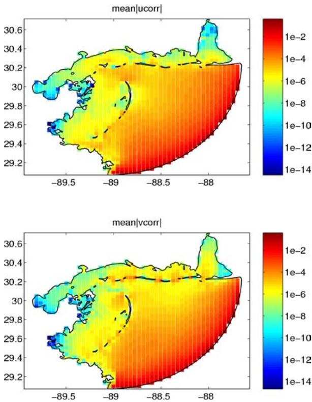
Fig. 10. Mean absolute values of the modulus of the complex correlations for the  $M_2$  tide E-W and N-S velocity components.
