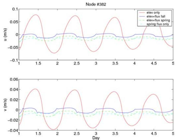
Fig. 11. Pearl River E-W and N-S velocity components at station #382 for three forcing conditions in spring and one in fall.
