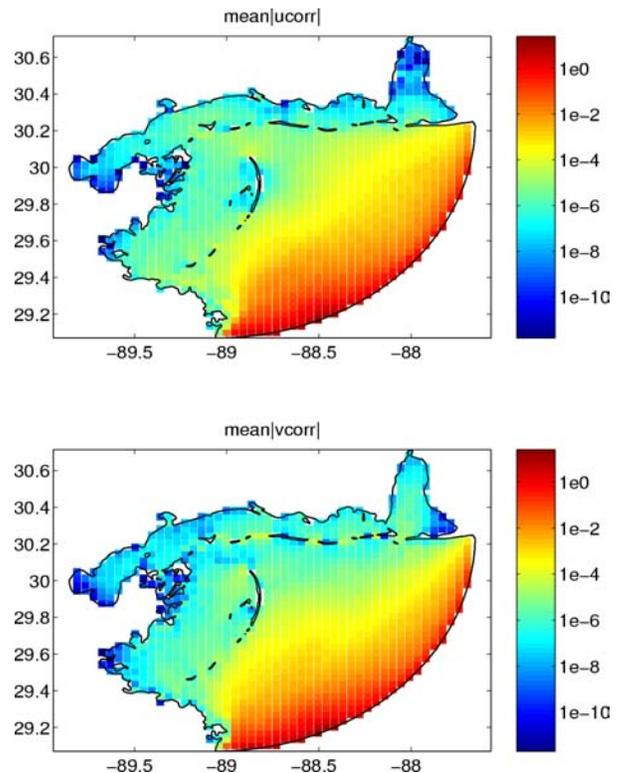
Fig. 9. Mean absolute values of the modulus of the complex correlations for the  $O_1$  tide E-W and N-S velocity components.
