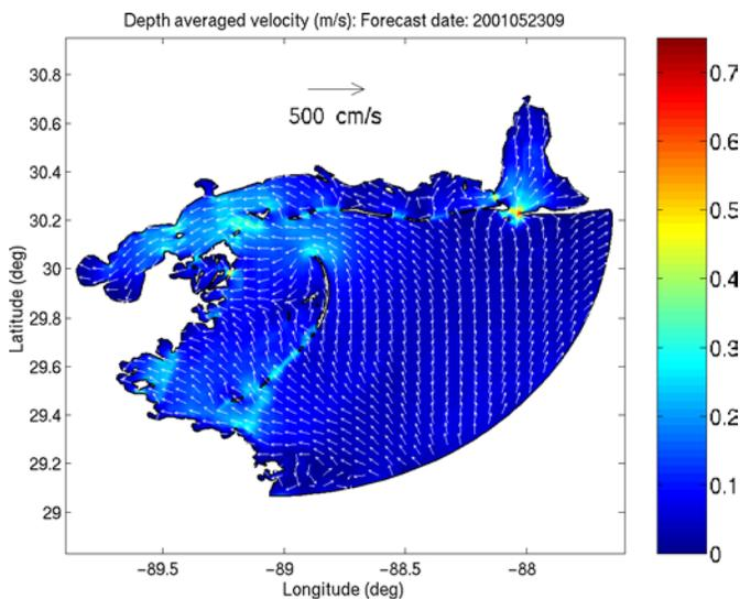
Fig. 8. ADCIRC computed currents on May 23, 2001 09Z forced by NDBC buoy winds and tides. Current magnitudes are contoured; directions are indicated by the arrows.
