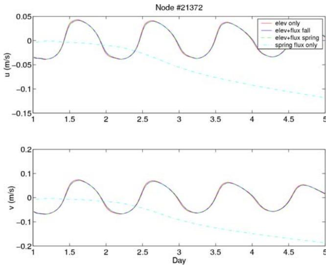
Fig. 13. Pearl River E-W and N-S velocity components at station #21372 for three forcing conditions in spring and one in fall.
