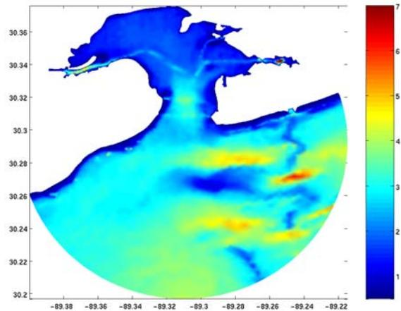
Fig. 2. Bathymetry of the Bay St. Louis model. Bathymetry contour range from 1 to 6 meters.
