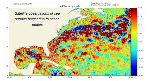
Satellite altimeter systems measure the ocean surface height with accuracy to a few centimeters. Ocean eddies have scales of tens to hundreds of kilometers, and these features persist for weeks to months. The sea surface height reflects changes in temperature deep within the ocean
