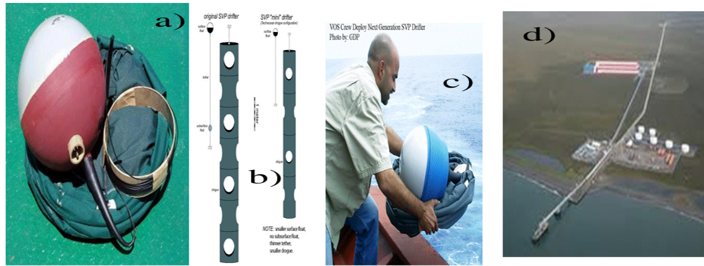
Figure 3. a), b), c) Sea Surface Drifters and a typical way of its deployment. d) Red Dog Port terminal in the Chukchi Sea: serves as a gate for loading zinc ore onto ships that steam toward Japan through the Bering Strait. e) Dots show shore locations 1) Pt. Hope, 2) Red Dog, 3) Little Diomed and yellow stars show drifter launch locations.
